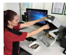
Portable energy dispersive X-ray fluorescence spectrometer (ED-XRF) for preliminary elemental analysis
